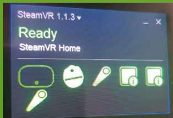
7. To change VRGO binding options open the drop down menu from the SteamVR desktop application and select devices>controller input binding. This can be done in VR while wearing the HMD also.
